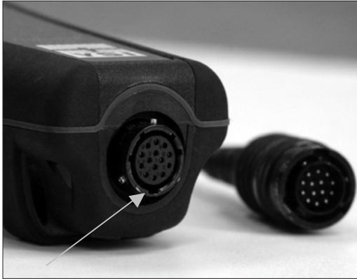
Figure 5. Note the keyed connector. The cable and instrument connectors can only be mated once the keyed sections are properly aligned.
